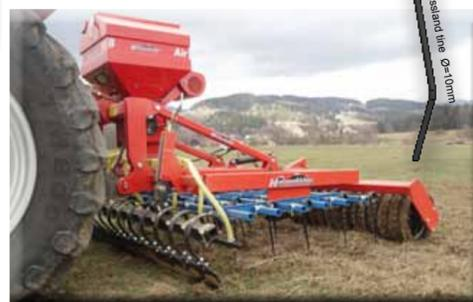
Heavy Vertikator 3m working width in use
