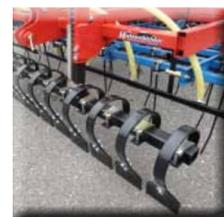
Single mounted, spring-loaded leveling plates
