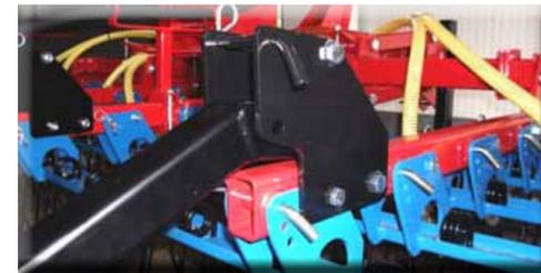
New constructed roller suspension
