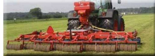
Vertikator 6m working width with pneum. Seeder „Air 16“
