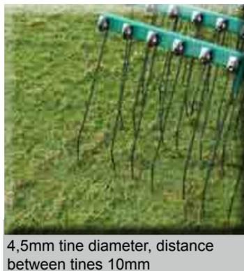
4,5mm tine diameter, distance between tines 10mm
