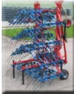
12m Harrow in transport position (shear folding).
