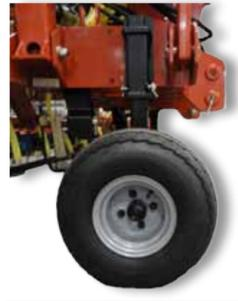
Adjustable wheel hubs with screwed and tapered roller bearings.
