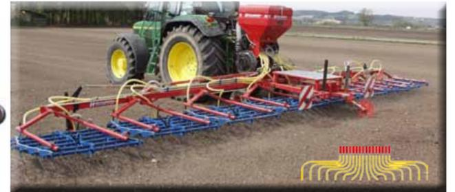
Harrow, 12m working width with pneum. seeding machine „Air 16“
