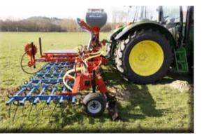
Vertikator "Hegler Sepp", strong version, 6m working width
