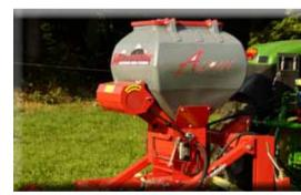
The special pressure rollers behind the harrow and the pneumatic Seeding machine complete the perfect pagination loose pasture renewal. The more divided pressure roller presses the seed and results in good soil contact. The pressure roller is characterized by excellent ground, even on the most difficult terrain. Even in wet conditions - no sticking of the rolls
