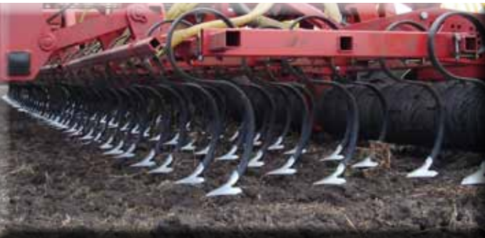
Equipped with cultivator tines (H90) and duck foot shares or small shares
