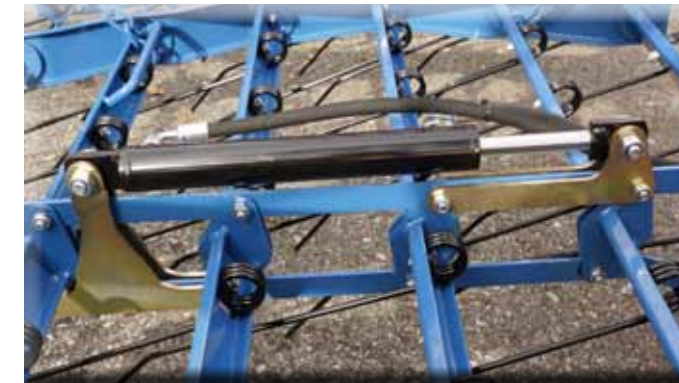
Cylinder for hydraulic tine adjustment
