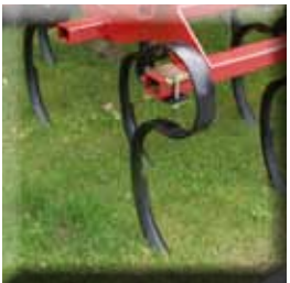
Equipped with „Hercules“ tines and small shares
