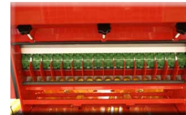
Seed roller with single outlets
