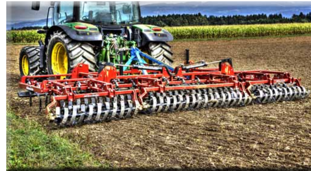
5,50m cultivator with rotor spring roller
