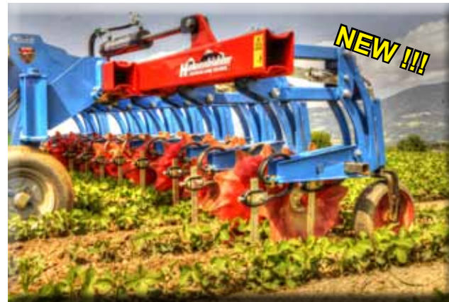
New designed 9-row interrow cultivator only possible front mounting
