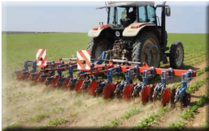
12-row sugar beet interrow cultivator with protection discs
