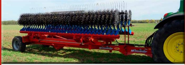
Rotary-Hoe 12,20m working width in working position and transport position
