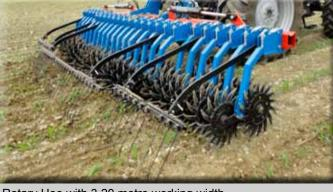
Rotary Hoe with 3,20 metre working width
