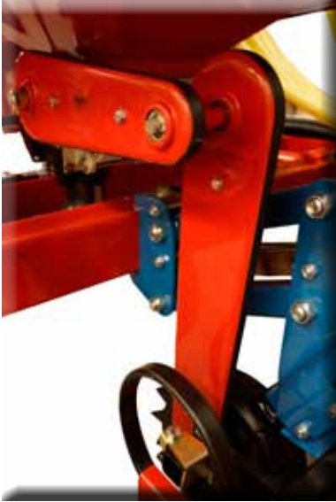
drive cassettes about metering wheel
