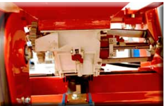
seed outlet with discharge flap share
