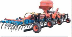
Harrow, 6 m working width, with pneum. seeder, Grassland sheets of reinforced design
